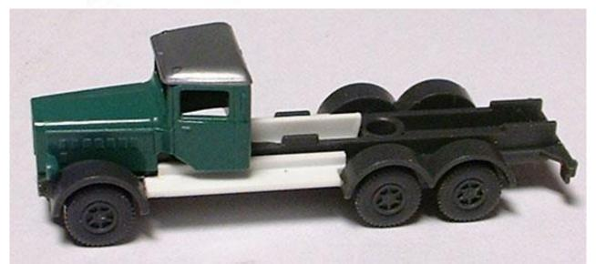
3. The wrecker bed is fabricated, and wheel wells are formed with the help of a rotary cutter.
